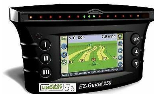
Figure 4. Example of a more sophisticated lightbar (EZ-Guide 250 de Trimble https://trl.trimble.com/docushare/dsweb/Get/Document-699587/Sistema%20EZ-Guide%20250%20-%20Hoja%20de%20datos%20-%20Español%20-%28Spanish%20EU%29.pdf multiconstellation)
