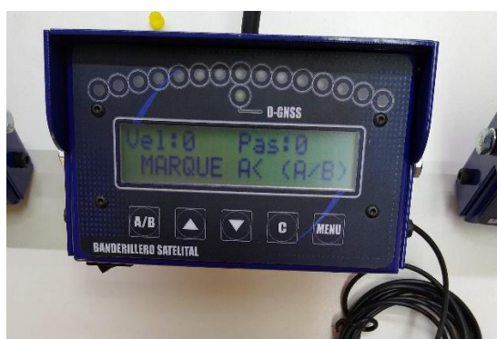
Figure 3. Example of a simple lightbar (Bandertbit by Artbitingeniería https://arbitingenieria.com.ar/banderillero.php )
