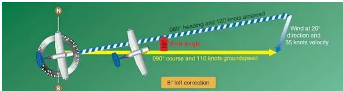
Figure 2: The principle of dead reckoning wind triangle
