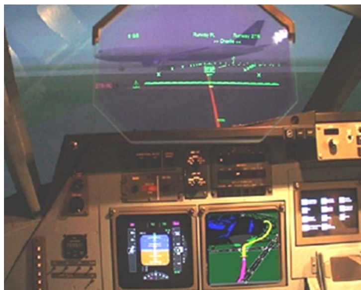
Figure 13: DGPS T-NASA HUD integrated within aircraft cockpit
